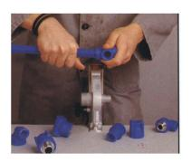
The welded connections are fully loadable after approx. 30 minutes.
