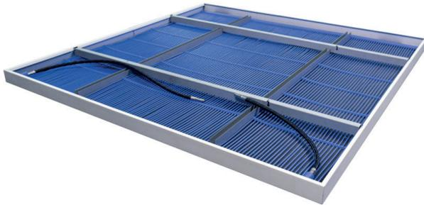
In the case of unperforated metal canopies the capillary tube mat is fixed directly on the metal and in the case of perforated metal canopies, which are usually covered on the inside with an acoustic fleece, it is fixed on the fleece, mostly with adhesive.
